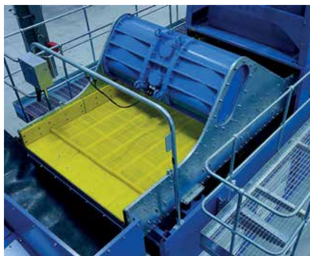
Galvanising is not an option. It's the Infinity standard - and it ensures the longest working life for your Infinity screen.
